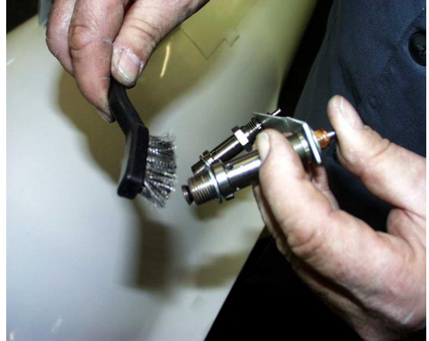
Picture 2 Cleaning of the decompression valves
